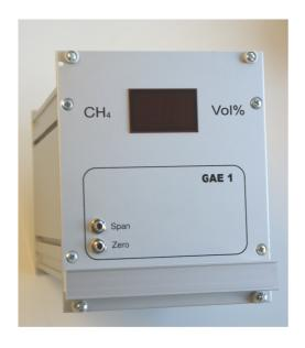
The gas analyzer GAE is a non-dispersive infrared-photometer (NDIR). It records the absorption of infrared rays, caused by the measuring gas. The wavelengths of the absorption bands characterize the type of gas, whilst the intensity of the absorption is a measurement for the concentration of the measuring components.
